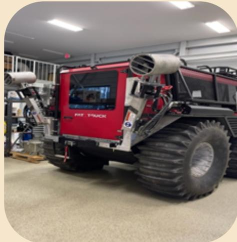
Fat Truck fitted with thruster for water crossings
